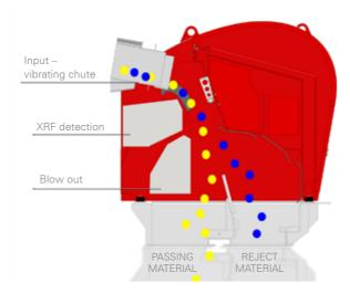
The **REDWAVE XRF-M** chute innovation is a further development of the established REDWAVE XRF belt design, which has been successfully in operation worldwide for many years in e.g. glass recycling plants. The **REDWAVE XRF-M** was specifically designed for the metal recovery industry. It combines the established XRF-technology with the superior chute design, which drastically improves the detection efficiency and, therewith, the product purity.
