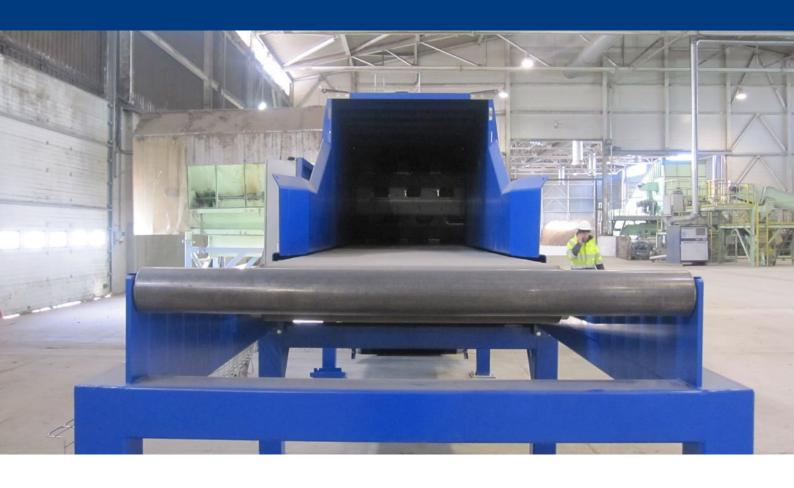
The solution was simply to install the ReTec bale-opener in front of the existing drumscreen-opener, and convert it to a conventional drum-screen. With the SRF completely loosed, the screen can now very effectively screen the wrapping from the fluff. The output is very clean and homogenous flow of fluff, and the waste fraction is very pure, i.e. contains very little SRF.
